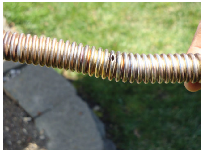
CSST with Jacket Removed Showing Typical Lightning Damage.
